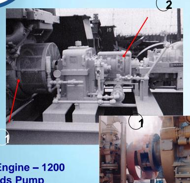
**Combustion Engine – 1200** hp / Goulds Pump
